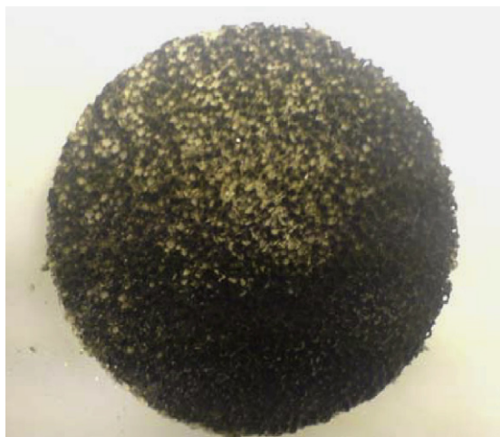
Fig. 17. Zirconia-treated alumina foam from autothermal reforming of jet A-1, 18.5 g/min, after final experiment.
